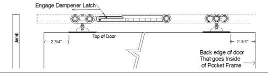
Move door, into wall of Pocket frame. (Double Check to Make sure no track screws are interfering with the Soft close Dampener trigger). Install the Activating arm stop into the track 2-1/4" from the jamb at the end of the track by hand. Be sure that arm is in the center of the track. Now slowly close the door to the jamb. Adjust Activating arm if needed to allow door to touch Jamb.
