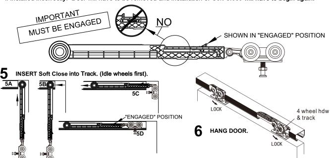
**SLIDE** door away from end of track (*check to make sure all track* screws are flat against track) and install Actuator Arm into track, with back of Actuator Arm 2-1/4" (57mm) from Jamb.
